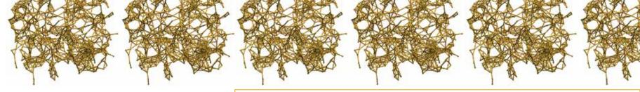
Dendrite crystals like these can short out batteries and even trigger explosions under certain conditions. Research at the School of Natural and Behavioral Sciences is focused on creating a cheaper, aluminum-based battery similar to those made of lithium, an element whose chemical properties stall dendrite growth.
